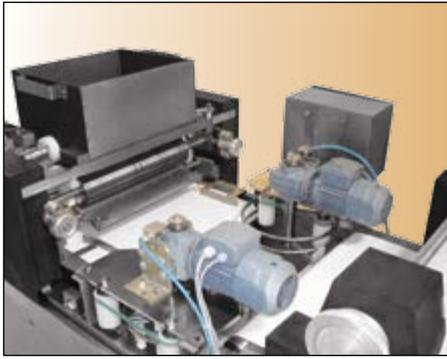
Cream spreading machines spread an exact amount of cream onto the wafer sheets and automatically stacks the requested number of spread sheets together with the un creamed top sheet into a wafer block. A thermostat allows to heat the cream spreading roller as well as the counter-roller up to an exact temperature. The speed of the two rollers and of the spreading belt can be steplessly adjusted independently of each other.
