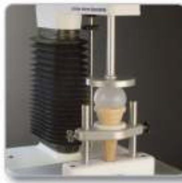
Ice Cream Cone Strength Assesses the structural strength of ice cream wafer cones under compression, simulating likely conditions of use.
