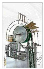
This machine is used to transfer wafer sheets\*\* or wafer books from one level to another. (This catalogue describes the details from one floor to another, for wafer books.) It can be customized for
